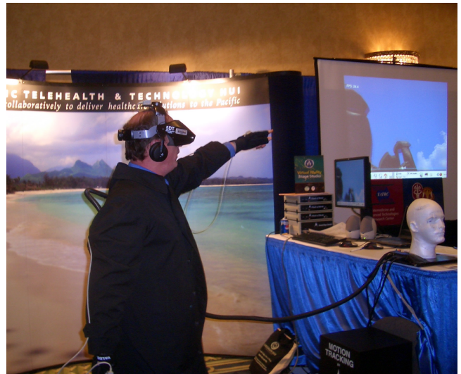
Figure 4: A virtual traveler is negotiating his way between large stone pillars, using steering-by-pointing technique. The first person view is also projected onto a screen (top right).
