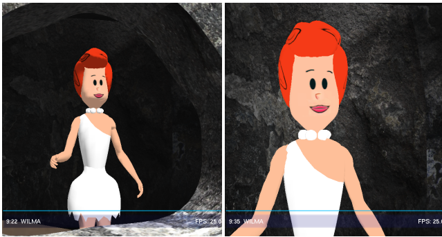
Figure 6: The travel system can automatically select between outdoors lighting (left, directional sunlight) and indoors lighting (right, head-mounted spotlight), by checking values in the blue channel of the terrain map. All pixels in elevation map inside the building have blue values set to 0.
